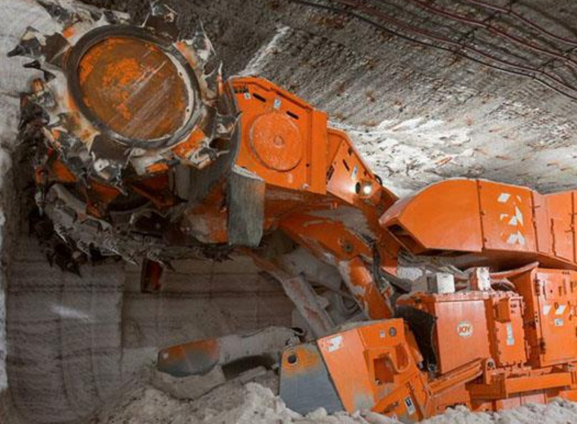
Efficient "continuous mining" technology applied at an underground salt mine
